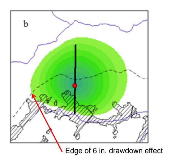
Drawdown distribution simulated using detailed MODFLOW model (courtesy of USGS)
